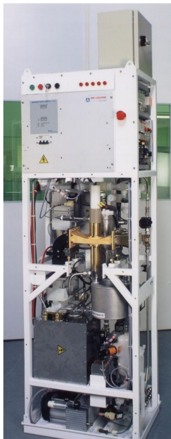
First Air Liquide prototype assembled to eliminate green-house gases currently used in micro-electronics fabs (chips manufacturing), built according to Moisan's team indications
